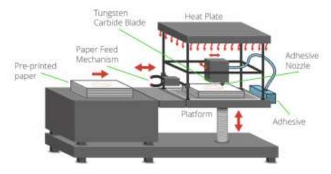
SDL is a proprietary 3D printing process developed and manufactured by Mcor Technologies. There is a temptation to compare this process with the
