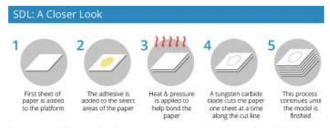
SDL is one of the very few 3D printing processes that can produce full colour 3D printed parts, using a CYMK colour palette. And because the parts are standard paper, which require no post-processing, they are wholly safe and eco-friendly. Where the process is not able to compete favourably with other 3D printing processes is in the production of complex geometries and the build size is limited to the size of the feedstock.
