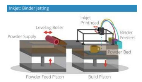
Binder jetting: where the material being jetted is a binder, and is selectively sprayed into a powder bed of the part material to fuse it a layer at a time to create/print the required part. As is the case with other powder bed systems, once a layer is completed, the powder bed drops incrementally and a roller or blade smoothes the powder over the surface of the bed, prior to the next pass of the jet heads, with the binder for the subsequent layer to be formed and fused with the previous layer.
